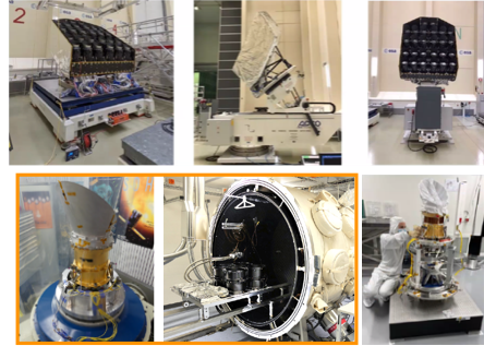
PLATO TOU Structural & Thermal Model (STM) on UBE shaker (left) TOU Flight Model (FM) mechanical parts inside UBE thermal chamber. Credit: UBE
