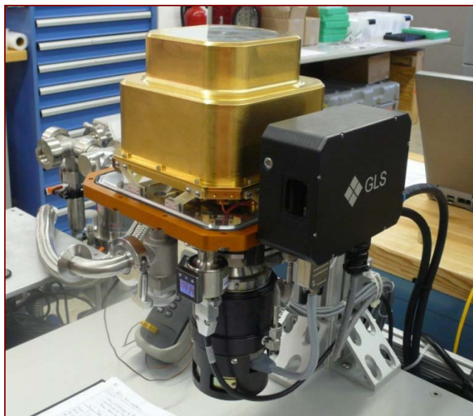
Figure 3. Internal view of the SCC-g2 cryostat with radiation shield visible surrounding the inner sanctum. Please see text for component descriptions and dimensions.
