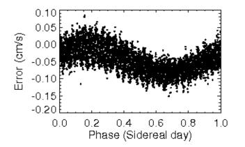
Figure 6: (Wright & Eastman) Comparison of the barycentric correction generated by TEMPO2 versus that generated with our code using the method described in this paper over a 14 year period. The residuals have an RMS of 0.037 cm/s and a peak to peak difference of 0.24 cm/s with no long term trend. The residuals phase with the sidereal period, suggesting that the dominant shortcoming of our code is in our treatment of the Earth's orientation.
