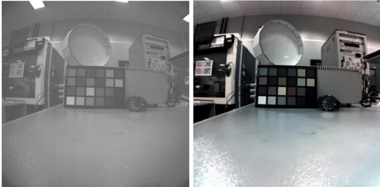
Figure 2. Left: Raw image taken by the RadCam/JMC PFM01 in the laboratory. The square patterns of the CFA are visible. Right: Final image after complete processing with the RadCam IPS.
