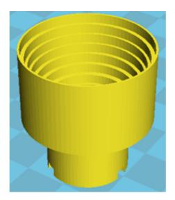
You also need supporting structures when you print the «Buffle». Print the «Buffle» in the position you see on the picture above.
