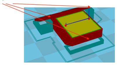
The «Backpart» is aligned and connected to the «Tube Assembly» through two small connectors.
