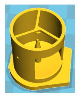
As during the printing of the «Spacecraft» part you also need to print supporting structure when printing the «Tube Assembly». Print the «Tube Assembly» in the position you see on the picture above.
